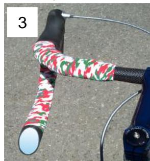
3. Fasten in position with plastic tape. Wrap bar tape around the mirror up to the edge as shown.
