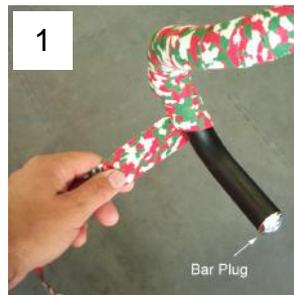
1. Unwrap about 10 cm (5 inches) of bar tape. Insert a bar plug into the end of the bar.
