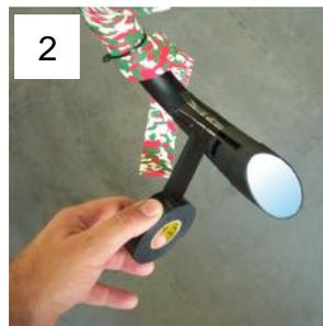
2. Place the rubber flaps OVER the end of the bar. Get on the bike in riding position, then position the mirror so you can see behind you as shown.
